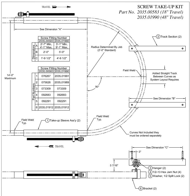
**DESCRIPTION:** The 2035 Screw Take-up Kit IS used in place of the Framed Take-Up (2035.01687) or when non standard curves are being used (anything other than a 2'-0" radius), or where the track spread is greater than 4'-0" (14'-0" max.). The 90° curves are not included and must be ordered separately The Screw Take-up Kit is finished with R-W standard baked enamel powder coat paint.
