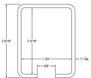
**DESCRIPTION:** The standard 2035.00471 track is a tubular section formed from 3/16" plate steel and is available in 10-foot lengths. A lighter weight, 11gauge (2035.00804) is also available. The track is finished with R-W standard baked enamel powder coat paint. Unpainted and stainless steel track are also available.
