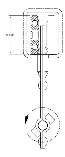
**DESCRIPTION:** The Four-Wheel Carrier is used for "Safe-Rail" applications. The carrier is equipped with hardened steel thrust rollers. The machined wheels are 2-1/8" in diameter and have a full compliment of steel ball bearings. The carrier side plates are zinc plated.
