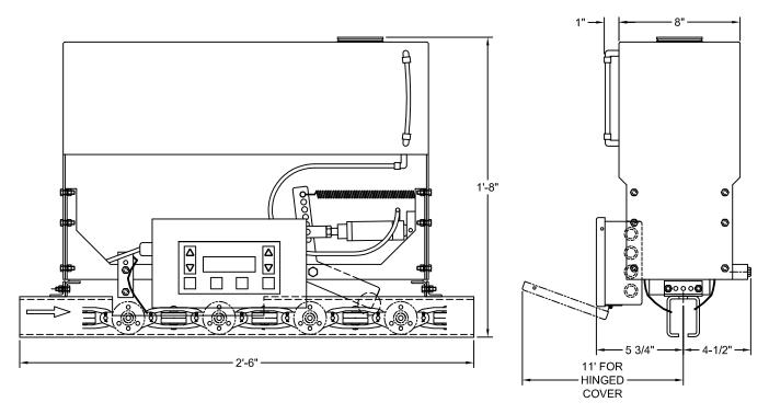
**DESCRIPTION:** The 2035.02893 Lubricator is designed to precisely lubricate the critical bearing points of the conveyor chain. The lubricator has five ejector tubes to precisely dispense the lubricant into the vertical and lateral wheel bearings along with the vertical link pin and roller. The unit has a micro-prossesor to accurately control the amount of lubricant that is dispensed.
