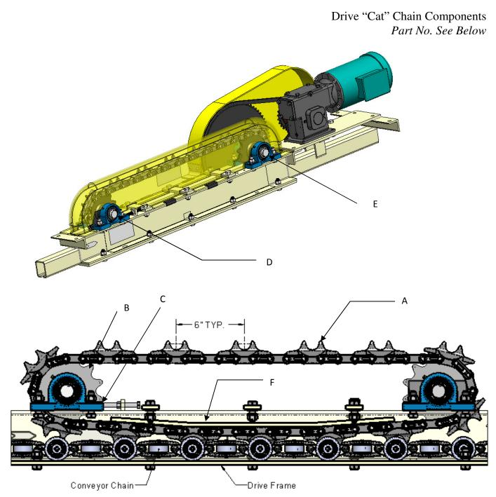
**Description:** The drive "Cat" chain transmits the power to the conveyor chain.
